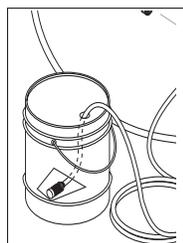
**STEP 2:** Use detergent designed specifically for pressure washers. Household detergents could damage the pump. Prepare detergent solution as required by manufacturer. Fill a container with pressure washer detergent. Place filter end of detergent suction tube into detergent container.
