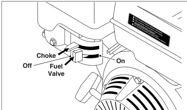
**STEP 6:** Slide the fuel valve lever to the "ON" position. When the engine is not in use, leave the fuel valve in the "OFF" position.
