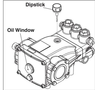
**STEP 2:** Remove shipping cap and install oil dipstick. Check pump oil level by using dipstick or observe oil level in oil window (if equipped). Use 40 wt. non detergent oil.
