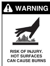
**WARNING:** Risk of injury. Hot surfaces can cause burns. Use only designated gripping areas of spray gun and wand. Do not place hands or feet on non-insulated areas of the pressure washer.
