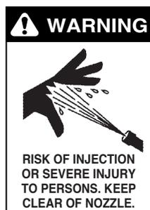
**WARNING:** High pressure developed by these machines will cause personal injury or equipment damage. Keep clear of nozzle. Use caution when operating. Do not direct discharge stream at people, or severe injury or death will result.
