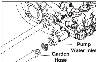
**STEP 7:** Check inlet filters, remove debris, then connect the garden hose to pump water inlet.
