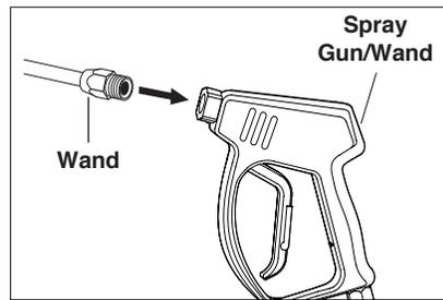
**STEP 2:** Attach wand to spray gun using teflon tape on wand threads.
