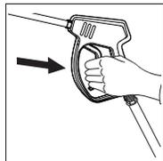
**STEP 4:** With the engine running, pull trigger to operate machine. Liquid detergent is drawn into the machine and mixed with water. Apply detergent to work area. Do not allow detergent to dry on surface.
