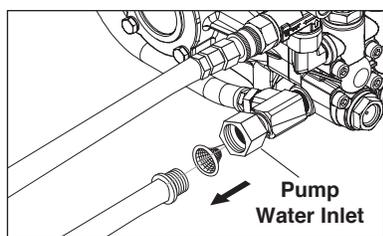
**STEP 5:** Disconnect the garden hose from the water inlet on the machine.
