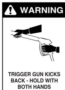
**WARNING:** Grip cleaning wand securely with both hands before starting. Failure to do this could result in injury from a whipping wand.
